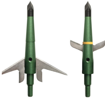
Figure 2c. #207 Sw Hacker® (FL Outdoors), 100 grain mechanical broadhead. On the left, the retention band is released and the retractable blades are fully deployed. On right, the retention band is intact and the blades are retracted. Image downloaded from https://floutdoors.com .
